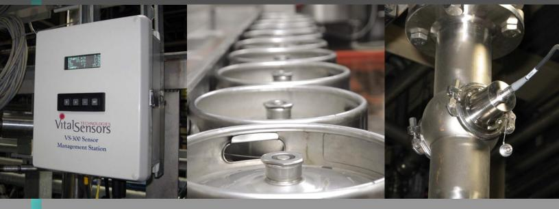
**VitalSensors Technologies LLC** is the leader in innovative, inline instruments for the food, beverage and pharmaceutical industries. The VS-3000 Beer and Wine Monitor measures three concentrations and temperature simultaneously using one sensor.
